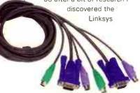
ProConnect KVM 2-Port Switcher — a dirt-cheap device for sharing one monitor, mouse, and keyboard between two PCs.
