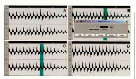
Fig. 2. (A) shows the original signal. In (B), the highest peak has been located and is about to be attenuated by -3 dB. (C) shows what happens after attenuation — it's now only a little higher than the other peaks. In (D), the overall signal has been normalized up to 0.00 dB. Note how the signal has a higher average level than in (A) — all the other peaks are higher than they were before — but there was no need to use traditional dynamics processing.
