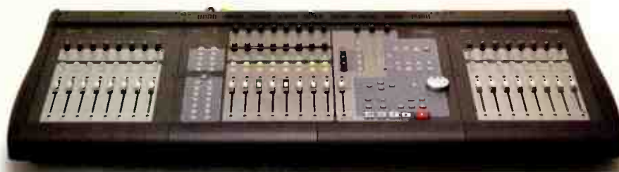
THE TASCAM FW-1884 (SHOWN HERE WITH TWO FE-8 EXPANDERS INSTALLED) OFFERS NEAR-UNIVERSAL CONTROL SURFACE COMPATIBILITY ALONG WITH 18 SIMULTANEOUS ANALOG/DIGITAL INPUTS AND OUTPUTS. AS A BONUS, THERE'S A 4-PORT MIDI INTERFACE BUILT-IN.
