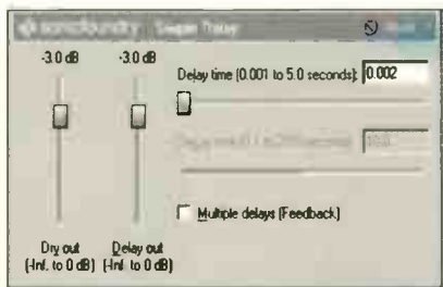
Sonic Foundry’s Simple Delay has been pressed into service as a comb filter.
