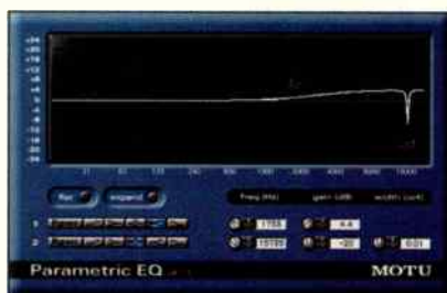
MOTU's ParaEQ 2-band is adding both a high shelf and a notch stage.
