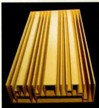
The RazorBlade from Primaacoustic is a quadratic diffuser; it spreads a precise series of different wells across a wall plane, and is designed to break up and scatter acoustic energy from 350Hz to 10kHz.
