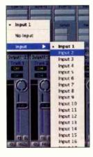
With the 828mkII, the first two ins are Mic/Guitar inputs 1 and 2. Logic labels them Input 1 and 2. That leaves Logic to label the 828mkII's Analog 1-8 as "Input 3-10." Confusing!
