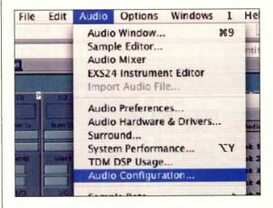
Within the audio configuration choose I/O labels from the View menu. Here you can select the "Long I/O Label" button for each input and type in a clearer name: "Mic/Guitar 1."
