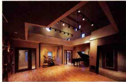
BiCoastal Music's massive live room has a 22' ceiling. The upper portion (above the soffit) is designed to be live, giving the room a natural reverb tail where desired.
