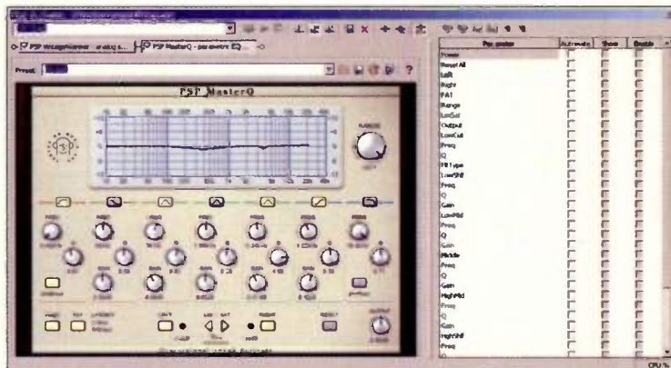
Fig. 3: Sound Forge's plug-in chainer allows creating chains of effects, and saving them (with settings) as presets.
