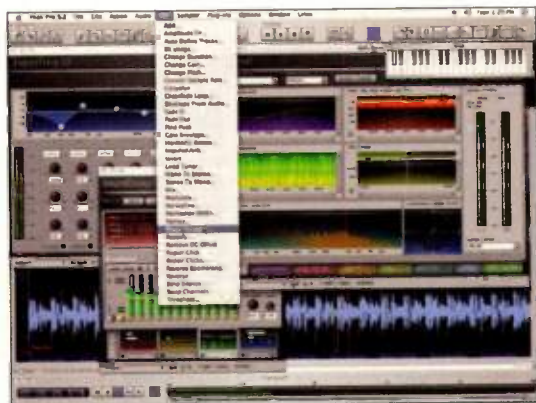
Fig. 1: The upper left shows the SuperFreq-10 equalizer; to the right is the Reveal suite of analysis tools. The generous DSP options are shown in the menu toward the middle of the screen, while SoundSoap Pro is behind it and to the left. The loooong meter is at the bottom, and just above it, one channel of the waveform view.
