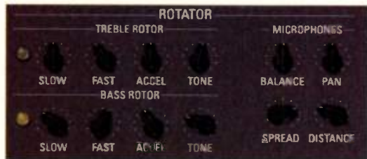
Fig. 2: Playing with the "spread" and "distance" setting of B4's rotating speaker simulator can lead to a fuller sound when miking its output.
