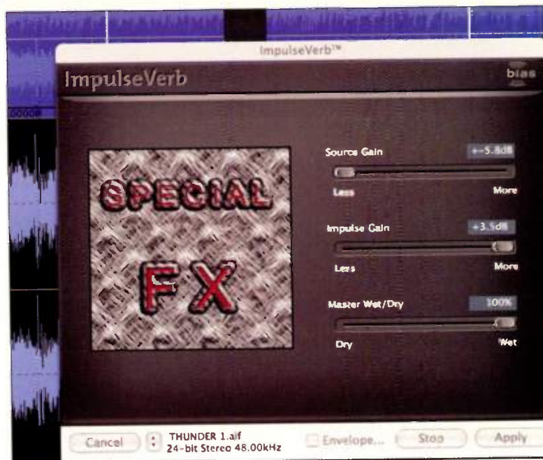
Fig. 2: Convolving sounds with unusual impulses, such as guitar bodies or even thunder (as shown here with BIAS Peak 5.2), can turn garden-variety found sounds into truly otherworldly effects.
