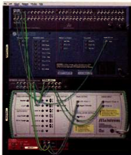
Fig. 1: A "Meta Patch" is the combination of various synth modules, connected together to create a new patch. This example uses Reason, Pro Tools, and a couple RTAS plug-ins.
