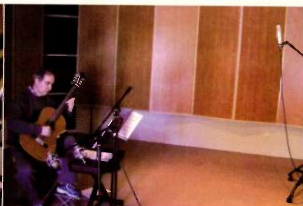
Fig. 2: Two Rode NT-2 overhead mics were located at some distance from the guitar, which captured the richness of the room but necessitated very quiet mics.
