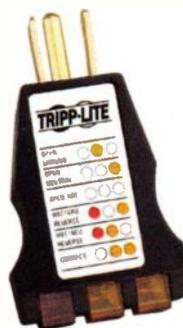
An outlet tester is a cheap addition to your live recording rig, but can spare you tons of unnecessary pain.
