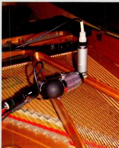
Fig. 1: An AEA R84 and a Neumann CMV563 placed in an M/S configuration.
