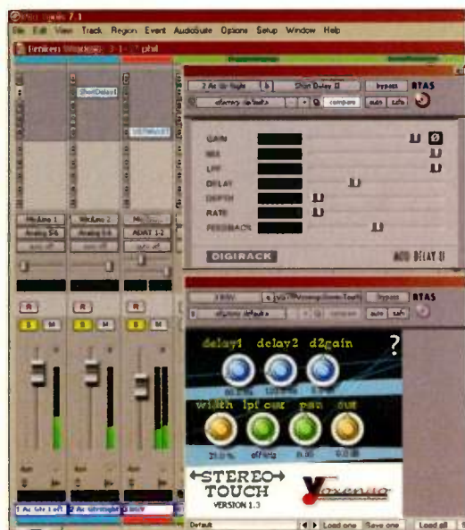
Fig. 1. Using delays and stereo-to-mono converters, along with judicious panning, can create new types of stereo placement effects.
