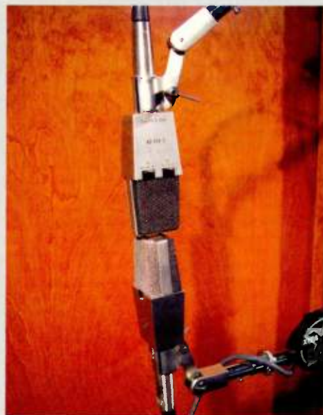
Fig. 2: Two condensers set up in M/S array.
