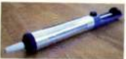
Fig. 2: Push down the plunger on a solder sucker, hold it over the connection, then heat the connection: Pushing the button creates suction that pulls the solder into the barrel of the sucker.
