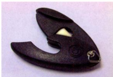
Fig. 3: Slide the cable into the cable cutter, then close the "jaw" for a clean cut. The blade is recessed, so it's virtually impossible to cut yourself accidentally.
