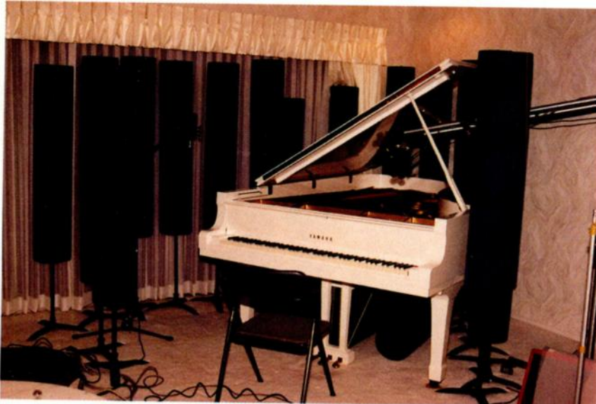
Fig. 1: Recording a duet in a living room. One large QSF lightly blends the vocalist and piano, while isolating them from the living room. Mics under the lid get QSF splash back.
