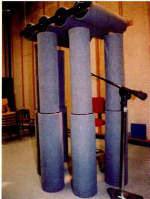
Fig. 3: This early QSF setup (circa 1987) uses an overhead QSF "cloud" to help hold in upward energy.
