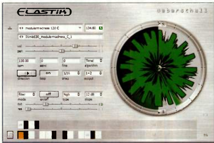
The Loop Eye provides a different way of defining loop start and end points.
