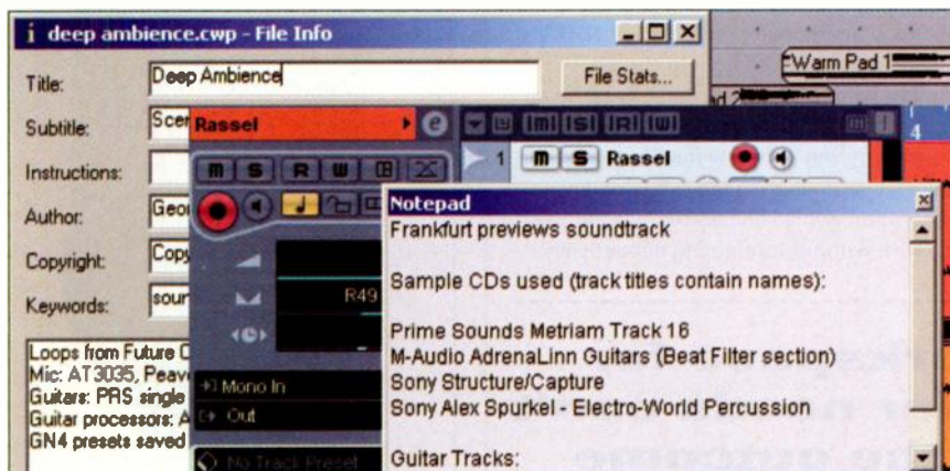
Fig. 1: Cubase (foreground insert) and Sonar (background) are just two of many DAWs with a notepad/info function for documenting sessions.
