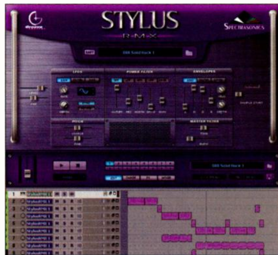
Fig. 5: The synth modules are on one page of the Stylus RMX interface. Below it, MIDI sequences have been dragged into the host program to create a drum part.
