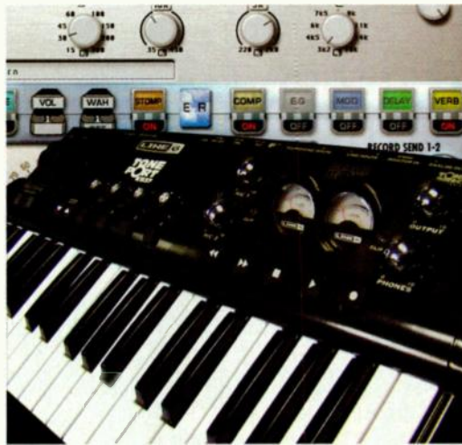
The KB37 superimposed on the GearBox software. This shows the software's effects chain and part of a mic preamp model above it.
