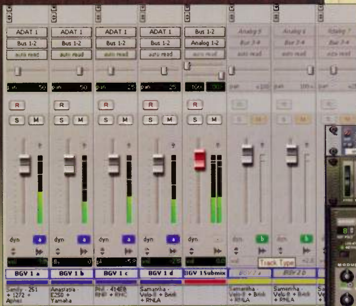
Fig. 1: By bouncing down tracks, it's possible to circumvent Pro Tools LE/M-Powered's 32-track limitation — without the downsides associated with track bouncing of the analog era.
