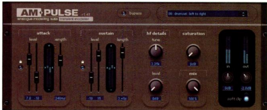
Fig. 2: The unusual, and highly effective, Am-Pulse analog modeling processor provides control over dynamics and transients.
