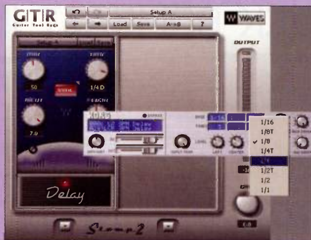
Ex 1: Two examples of delays with tempo sync. The foreground effect is the Korg MDE-X LCR delay, where the left, center, and right delays can have different sync values. The background effect is the Delay processor from Waves' GTR. Note that the Sync button is enabled, and the delay set to 1/4D (dotted quarter note).
