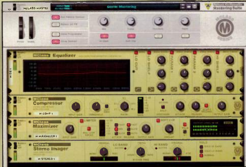
Fig. 3: Reason's MClass processors include an Equalizer, Compressor, Maximizer, and Stereo Imager. They're shown here placed in a Combinator.
