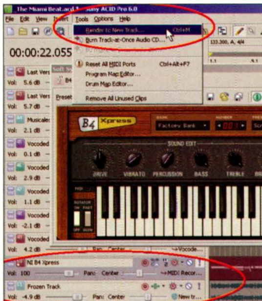
Fig. 3: Although Sony Acid 6 doesn't have a function called "freeze," the program makes it easy to render a soft synth's audio to a new track. Just solo the MIDI track driving the soft synth, select Render to New Track , and the soft synth audio shows up in a track added to the end of the project. You can then delete the soft synth to save CPU power.
