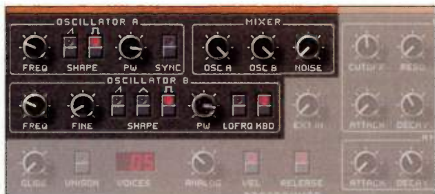
Fig. 4: Native Instruments' Pro-53 is one of many soft synths that provides pulse waveforms. Better yet, a pulse width control determines whether the pulse is narrow or wide.
