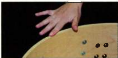
Fig. 1. Run your finger or palm along the bearing edge to feel for imperfections.
