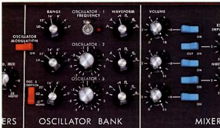
Fig. 1: This Arturia Minimoog V shot shows an archetypal Minimoog patch, with three oscillators set an octave apart via the Range controls. Note that the lowest and highest oscillators are tuned a bit off-pitch to add more sonic animation.
