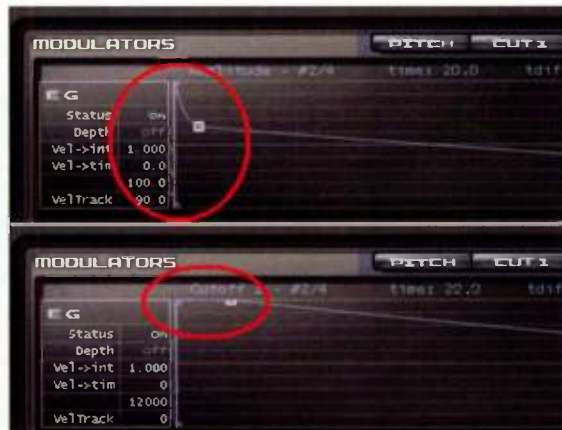
Fig. 2: The upper envelope generator picture from Cakewalk's Rapture shows a quick percussive decay that adds punch. The lower envelope setting achieves a more sustained punch effect by kicking the envelope full on for a couple dozen milliseconds.
