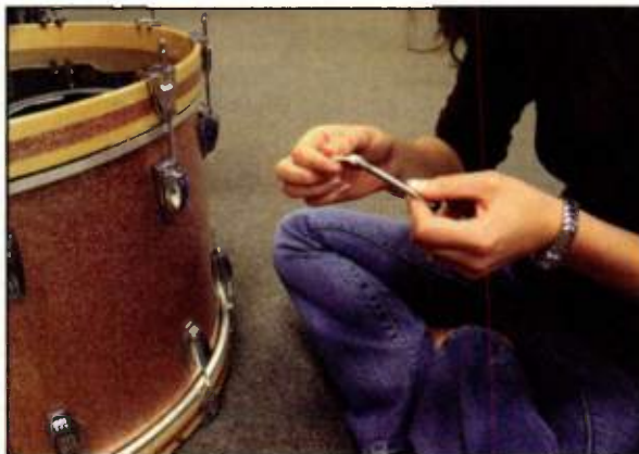
Fig. 3. Using a lint-free swab, apply a tiny amount of lubricant to each tuning rod.
