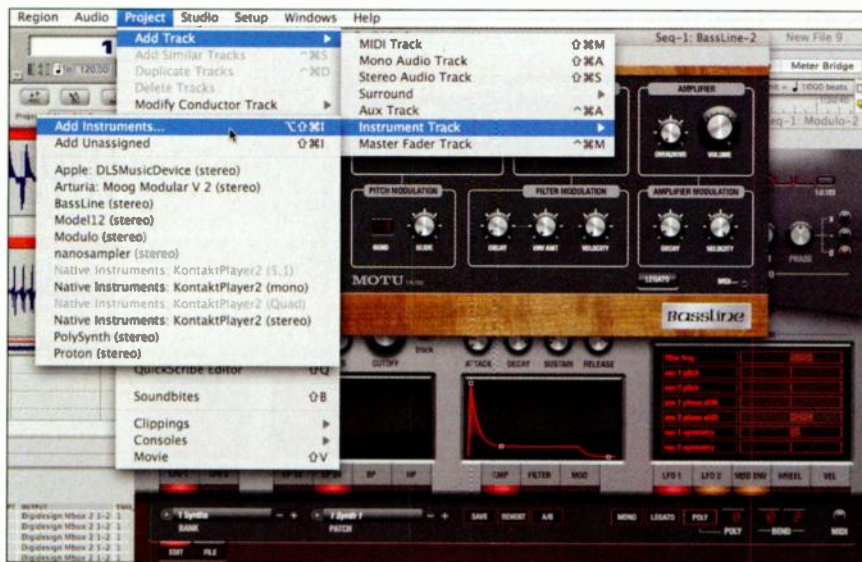
Fig. 1: Digital Performer already has the Modulo and BassLine instruments (included with the program) inserted. Another Instrument track is about to be created.
