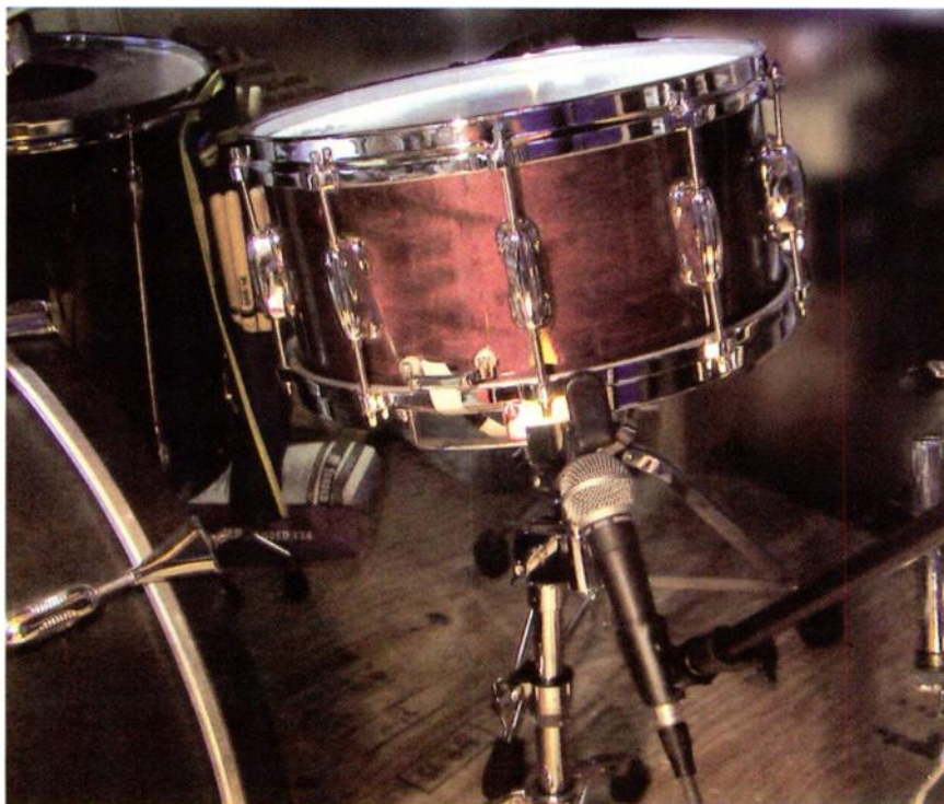
Fig. 1: A Slingerland snare's “under” mic. This is thrown 180 degrees out of phase compared to the “over” mic, which will be set up next. (Courtesy Brian Hardgroove, Public Enemy/EV2.)
