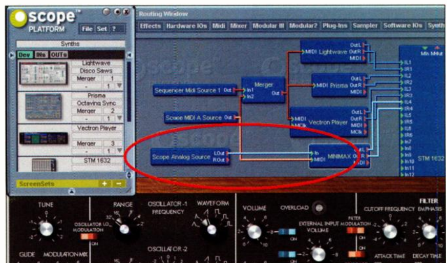
Fig. 4: The SonicCore Minimax is configured in Scope's routing window so that its audio input receives signal from an analog input (circled in red).
