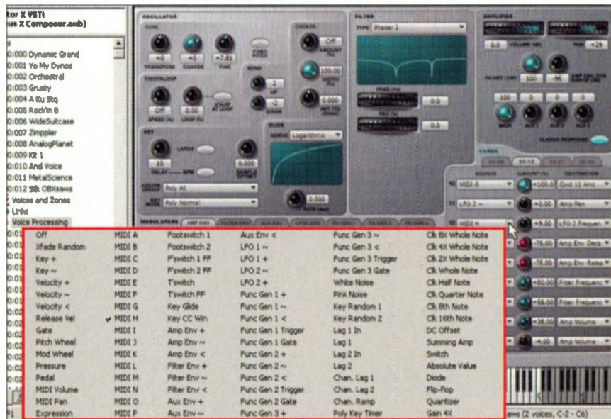
Fig. 6: E-Mu's Emulator X2 presents its modulation matrix as "software patch cords" that patch a modulation source to a modulation destination. This shows the list of modulation sources (outlined in red).
