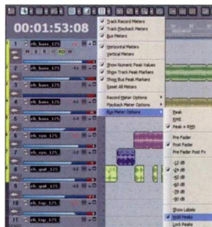
Fig. 2: Sonar offers a choice of horizontal or vertical meters in track view, as well as several options for tailoring the response, placement in the signal chain, and range.
