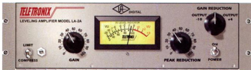
Many products, both hardware and software, pull double duties as compressors/limiters. Pictured are UA's software versions of the famed 1176 and LA-2A—two of the most highly rated compressor/limiters of all time.
