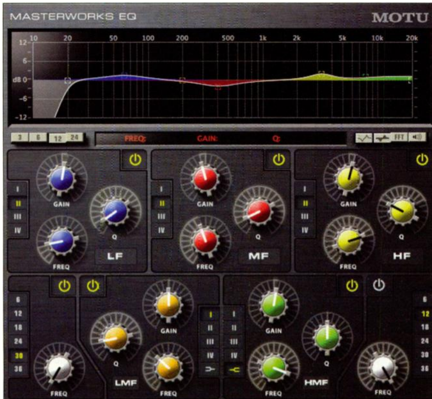
Fig. 2: Digital Performer's EQ set for a snare drum. Note the steep, low-cut filter below 20Hz, which helps get rid of unwanted subsonics. The high frequency shelf (colored green) adds a little "air."
