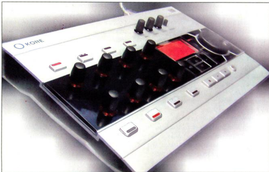
Fig. 7: Kore's hardware controller features eight switches and touch-sensitive controls to provide standardized control over plug-ins. It also allows fast preset searches.
