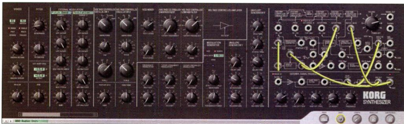
Fig. 5: Korg's MS-20 soft synth has been patched as an external processor for a drum loop. A trigger derived from the loop goes to the sample-and-hold (S/H) clock. The S/H input comes from an LFO, while the module's output controls the lowpass filter frequency. Meanwhile, the envelope follower output controls the VCA to let the signal through, and the Frequency to Voltage converter drives Oscillator 1 to add a sweeping oscillator effect along with the drums.
