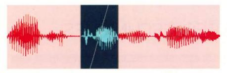
Fig. 4. Fading up from the plosive's point of impact can neuter the boom without damaging articulation or intelligibility.
