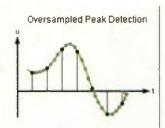
Fig. 1: An example of oversampled peak detection. Note how the reconstructed signal is higher in level than the individual samples would imply.
