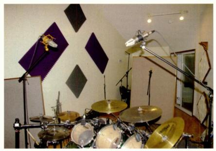
Fig. 1. The overhead mics are handled pretty traditionally to pick up the cymbals and the overall drum sound.
