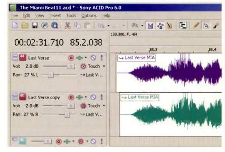
Fig. 1: Two copies of the same vocal track in Sony Acid. The lower track is delayed by about a 32nd note. Note that the upper track is panned 27 percent toward the left, while the lower track is panned 27 percent toward the right, to create a stereo effect.
