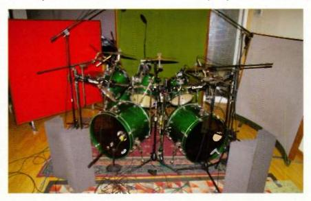
Fig. 3. Note the relationship between the mics and the kick drum heads.
