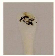
Fig. 1: Tape sheddings on the end of a Q-tip.
