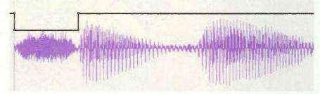
Fig. 2. Automating a dip in volume at the point of sibilance can help diminish the harsh "essss" sound.
