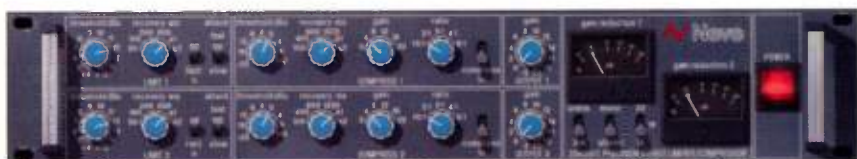
Fig. 2: Each channel of the Neve 33609 has a separate compression and limiting section.
