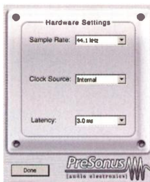
Fig. 1. Setting the latency in the Interface Control panel.
