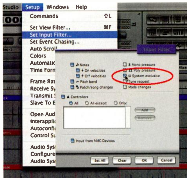
Like most programs, MOTU’s Digital Performer defaults to not recording sys-ex data. Going Setup > Set Input Filter brings up a dialog box where you can enable sys-ex recording.
