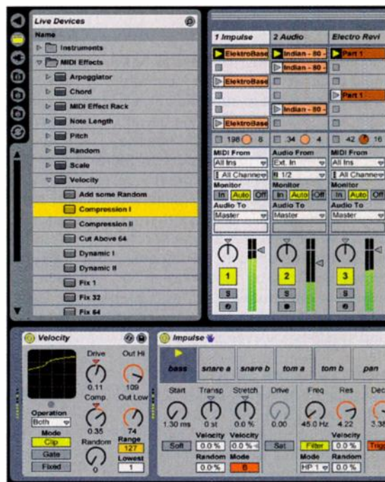
Fig. 1. Live's Impulse drum instrument is playing back a drum part; a Compression MIDI Velocity effect has been added before IMPULSE to even out the MIDI velocity values.
