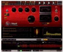
T-RackS 3 can be a plug-in or work stand-alone, as shown here. The Opto Compressor is just one processor in the chain; there are also two EQs and a brickwall limiter. Note the various displays for Spectrum, Phase, Peak, and Perceived loudness.
