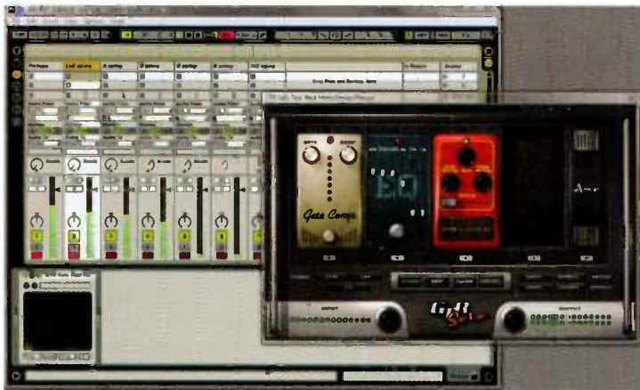
Fig. 1. This setup, based on Ableton Live as a host, layers and splits the six guitar strings to create a huge sound. The Waves GTR Solo patch shown toward the right provides octave division; using compression and EQ conditions the signal to deliver the cleanest possible octave division effect.
