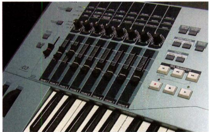
Fig. 6. Like many current hardware synths, Yamaha's Motif XS includes a control surface that works not only with synth parameters, but includes templates for providing realtime control over various programs.
