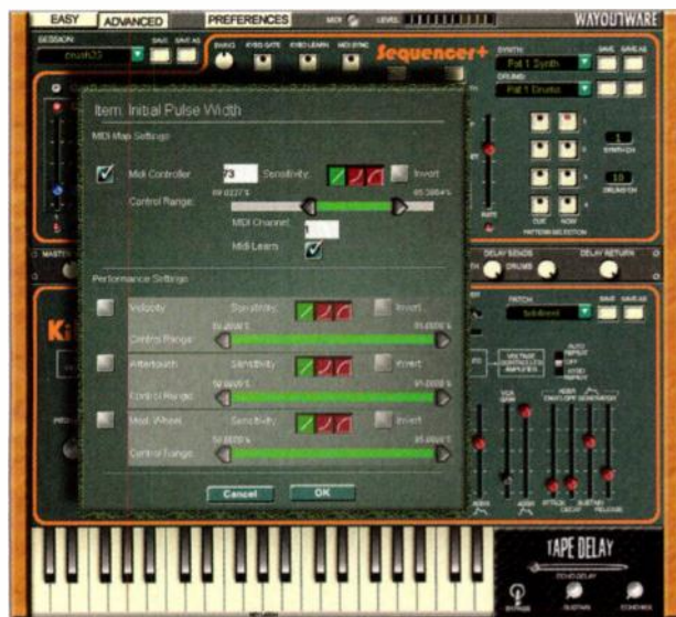
Fig. 7. KikAxxe from WayOutWare has a versatile control response. It offers MIDI learn, three different response curves, invert, and a range control where you specify the upper and lower limits; the linked hardware control covers the range you specify.
