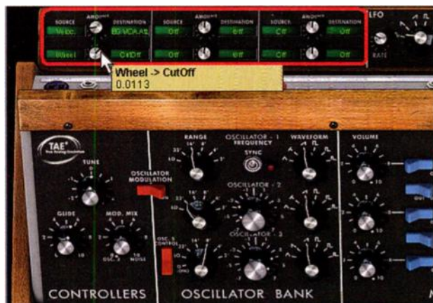
Fig. 8. Arturia's MiniMoog V includes a modulation matrix with six possible modulation sources and destinations. The Amount knob controls both range and polarity, depending on how it's turned: Counter-clockwise gives negative polarity, while clockwise gives positive polarity.
