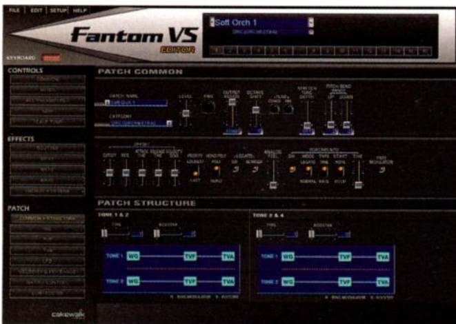
Fig. 3. The Fantom VS hardware is built into Cakewalk's V-Studio audio interface, but the GUI shows up on-screen as a virtual instrument plug-in.
