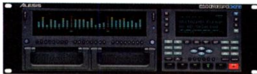
Fig. 6. The hard disk-based Alesis HD24 was conceived as a replacement for the ADAT, but has taken on a life of its own.
