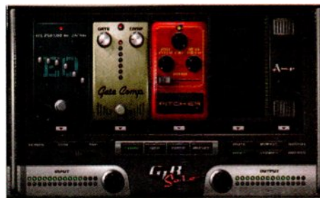
Fig. 1. Waves' GTR|Solo is set up for octave division on bass. The Pitcher module provides the octave division; its Mix control is set to divided sound only.
