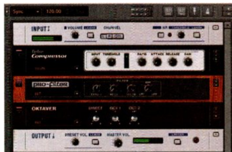
Fig. 2. Guitar Rig's Pro-Filter module is an excellent EQ for conditioning a bass signal before it hits the Oktaver.
