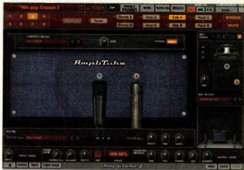
Two mics being set up on a cabinet, one close and centered, the other further away and on the edge of the speaker.
