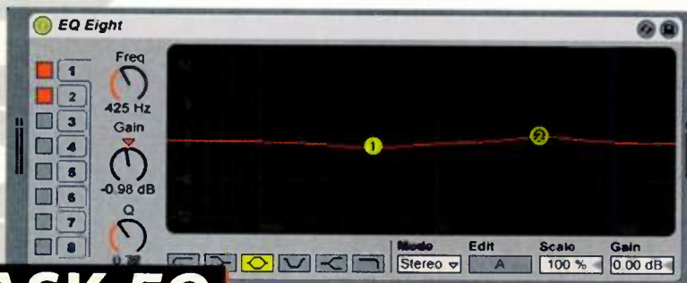
Live's 8-band EQ, which is inserted in the master bus, is cutting -1dB at 425Hz and boosting 1dB at 4kHz.
