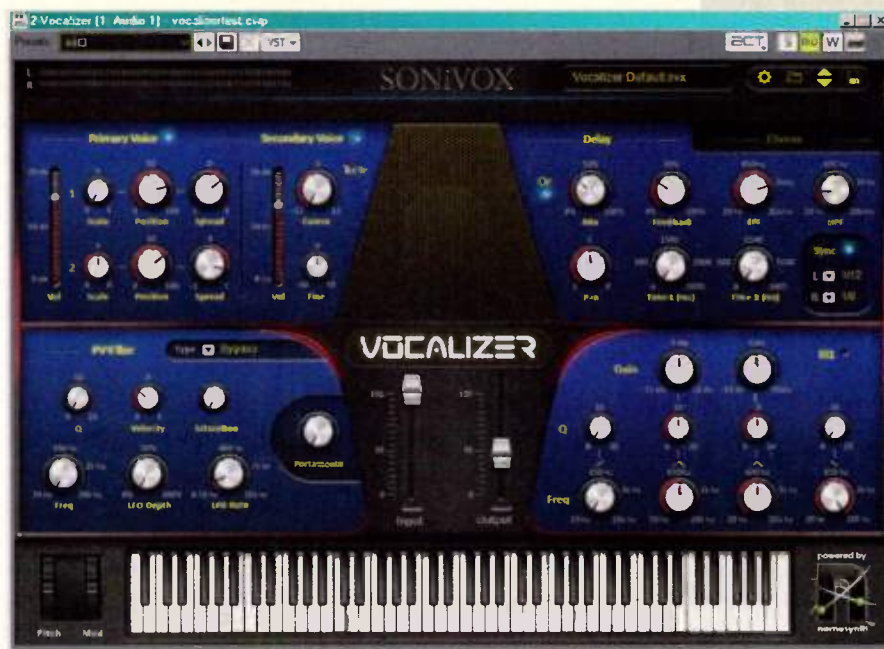
Fig. 1. The Vocalizer has an uncluttered layout; while most controls will be familiar, the Primary and Second Voice sections open up new possibilities for vocal processing.
