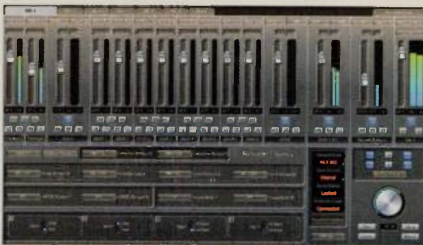
Focusrite’s Pro 24 DSP is just one of many audio interfaces that includes a mixer application for zero-latency monitoring.
