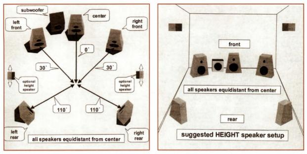
The Sony/Telare suggested arrangement for 6 channel SACD replay. Note the five identical and equidistant main speakers and optional "height" speakers. The spartan appearance of the room is closer to reality than most hi-bit manufacturers would have you believe, at least if quality is an issue.
