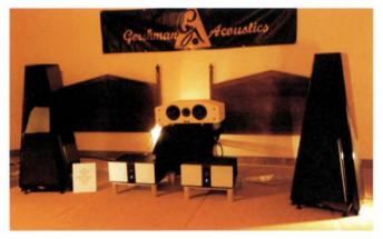
employing top-flight Scan drivers in a d'Appolito arrangement. The tapered, trapezoidal cabinets weigh around 75kgs each and feature external crossovers, loaded with such goodies as Hovland caps and Alpha-Core coils. The walls range between an inch and three-inches in thickness, with internal compart-ments further damped with a mix of lead-shot and sand, which
