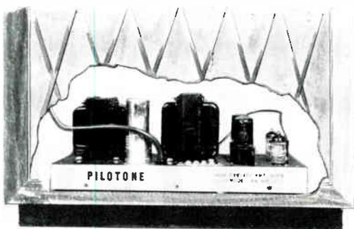
Fig. 4. The bottom of the speaker cabinet provides well-ventilated space for the amplifier, where it can be hidden readily
