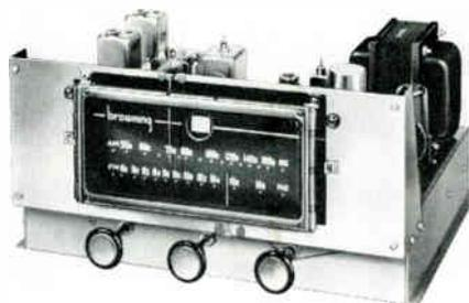
equipment at the rear of the chassis. FM circuits are of the Armstrong limiter-discriminator type. *Browning Laboratories, Inc., Winchester, Mass.*
