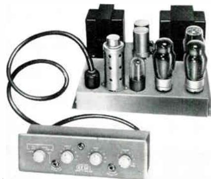
Fairchild, G. E., Pickering, and Sono-Tone. Connections are also provided for a tape recorder and tuner. The 10-watt amplifier, using KT-61 beam power tetrodes in push-pull is described as having .1% distortion at 1,000 cycles with 8 watts output. Dimensions of the amplifier: 11 ins. wide, 9 ins. deep, 6½ ins. high. The preamp: 9⅝ ins. wide, 2¾ ins. high, 3¾ ins. deep. *British Industries Corp., 164 Duane St., New York 13.*
