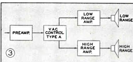
Thus it is possible to determine the optimum point, or points, *after your speaker system has been installed*. If, at any time, you want to experiment with other speakers, you can shift to any other crossover by merely resetting the calibrated control knob.
