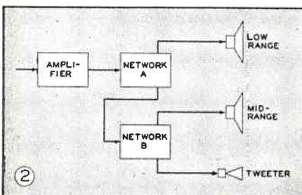
Coupler for the bass, a crossover of 175 cycles is generally used, or 350 cycles if the bass speaker is in a conventional cabinet.
