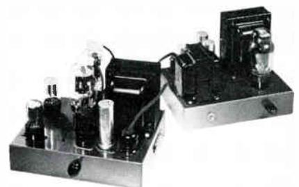
any dealer or mail order house. Construction is simple enough to be completed successfully by anyone who can handle a soldering iron. Instructions are also available for changing the regular Stancor Williamson-type amplifier to the new ultra-linear circuit. Performance of the new design is rated less than 1% total harmonic distortion at 1,000 cycles with 25 watt output. Chicago Standard Transformer Corp., Addison & Elston Sts., Chicago 18.
