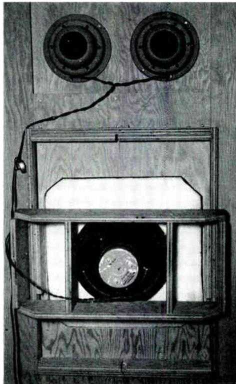
Fig. 4. Front view of the first experimental model, with the Styrocone speaker below, and two tweeters mounted above. This assembly was carried on a heavy piece of plywood, set in place of a closet door. This is a simple, ideal arrangement — where such a door is available. Fig. 5. Rear view, showing the support for the experimental speaker. Note that the cone is not supported at the edges
