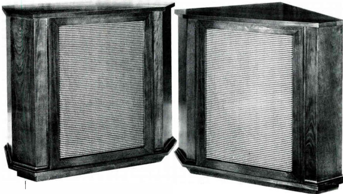
*While these cabinets are of moderate size, each contains a 20-in. Styrofoam speaker, and four tweeters. The latter are used to provide wide dispersal of treble tones. The cabinet at the left is intended to be placed directly against the wall; the one on the right fits into any corner. Both are built of solid mahogany, heavily braced to prevent vibration in any part of the case*
