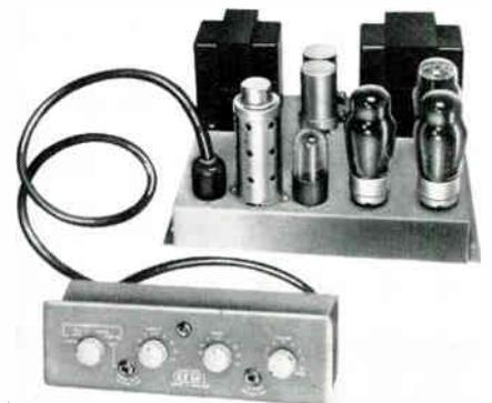
Fairchild, G. E., Pickering, and Sono-Tone. Connections are also provided for a tape recorder and tuner. The 10-watt amplifier, using KT-61 beam power tetrodes in push-pull is described as having .1% distortion at 1,000 cycles with 8 watts output. Dimensions of the amplifier: 11 ins. wide, 9 ins. deep, 6½ ins. high. The preamp: 9⅝ ins. wide, 2¾ ins. high, 3¾ ins. deep. *British Industries Corp., 164 Duane St., New York 13.*
