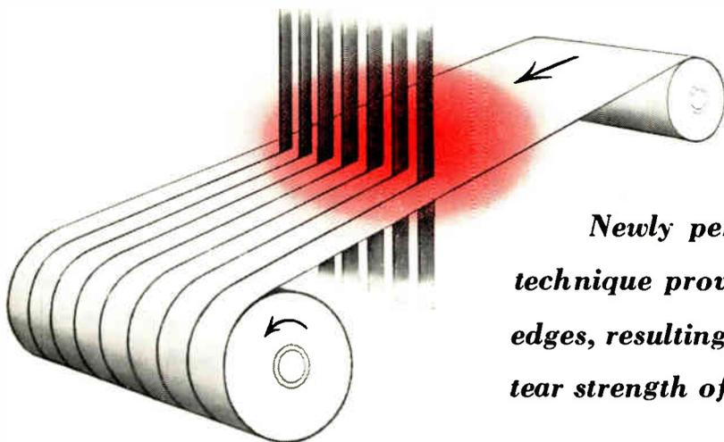
*Newly perfected thermal-slitting technique provides smoother, cleaner edges, resulting in increased break and tear strength of plastic base Audiotape*
