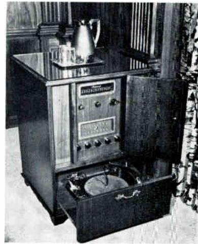
*Fig. 2. Connected to the cabinet in Fig. 1 is this compact control cabinet, containing the remote TV tuner, FM-AM tuner, and the phonograph in a drawer at the bottom*
