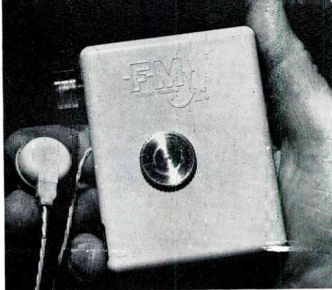
*Tuning knob for this tiny FM receiver is at the upper left, volume control and switch below. Antenna is at the top*
