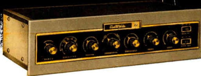
**Model A20CL Music Control Center and 20-watt Power Amplifier.** Features unique, exclusive "Presence" control. Response 20-20,000 cps.  $\pm 1.0$  db at rated 20 watts, 40 watts peak. Controls include Playing Selector, Loudness, Bass, Treble, Volume and Power, Phono-Selector. Power Amplifier utilizes Circlotron Circuit and Variable Damping Control. Low-boy styling. **Net, \$124.50**
