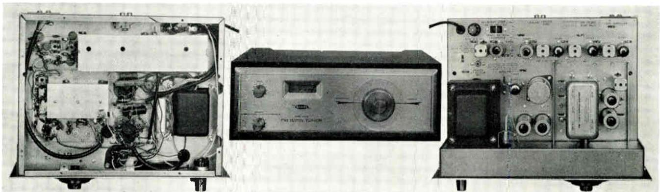
cent channels, a feature which is one of the important advantages of FM over AM. Tuning is done with a 3-section condenser. Silver-plated RF sections and shielding are designed to keep radiation below FCC requirements. Controls are for tuning, volume, and inter-station noise suppressor.
