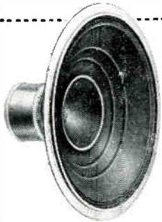
Norelco's twin-cone speakers are designed to meet the problem of high and low frequency dispersion in a single speaker. The large (heavy) cone is designed to produce good bass while the small (light) cone radiates higher frequencies.
