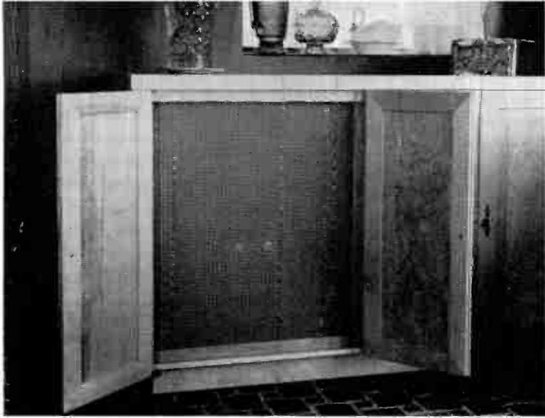
Fig. 10. The speaker in place. The base was removed from the enclosure, so it stands on the floor of the cabinet. This makes a more finished appearance
