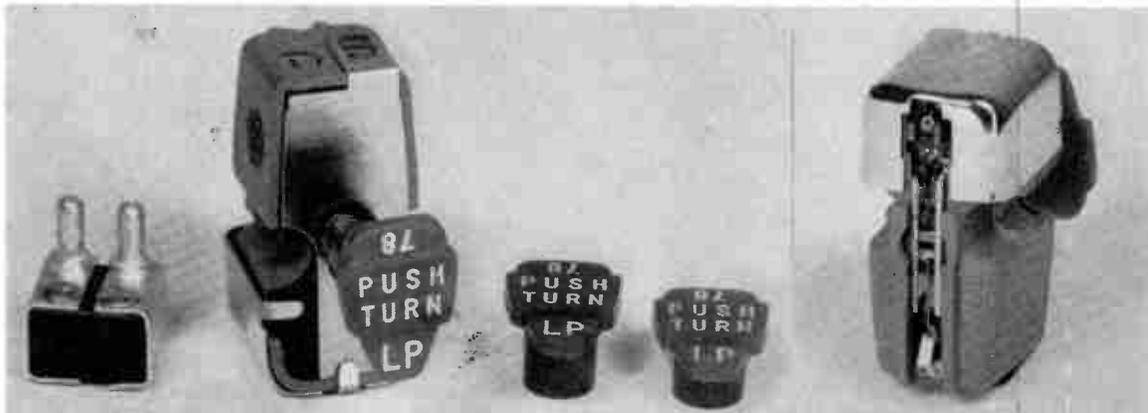
**Award No. 29. General Electric VR-II series pickups.** The new single-stylus and dual stylus types are a further improvement over the familiar RPX models. The body is narrower, the weight reduced by 27%, and the stylus 10% lighter. An electrostatic shield has been added to protect the pickup from outside electric fields which might cause interference.
