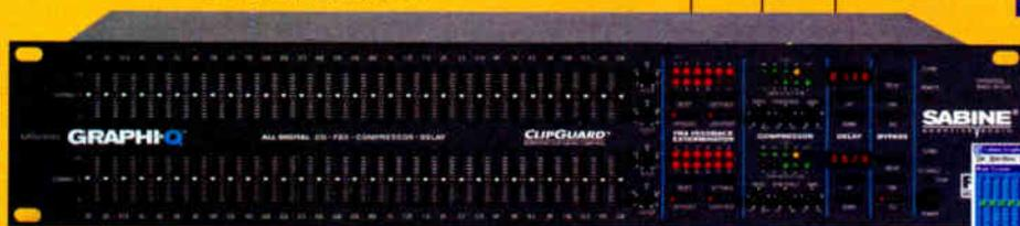
GRQ-3102 Front Panel Control (two in/two out)
