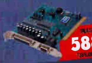
**DIGIGRAM • VX442** • Audio card • 6 simultaneous I/Os: 4 balanced analog 1/4Os and digital stereo I/O
