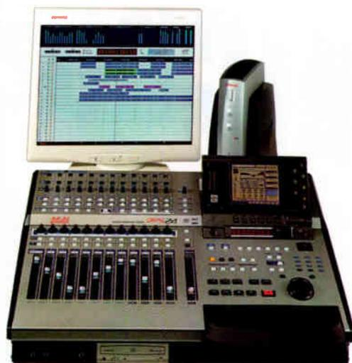
console's surface. The faders' feel and spacing were easy to move with my average-sized hands. There are four main layers: 12 mic/line input faders, HD tracks 1 through 12, tracks 13 through 24, and a fourth layer that is divided between eight group masters and four stereo effects returns. A fifth user layer provides access to effects sends to external devices, aux bus levels, stereo aux return to the L/R bus and three faders for MIDI control, but can be reassigned by the user.
