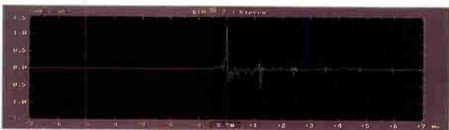
Fig. 2: HD-1's on-axis impulse response with Stewart MicroPerf
