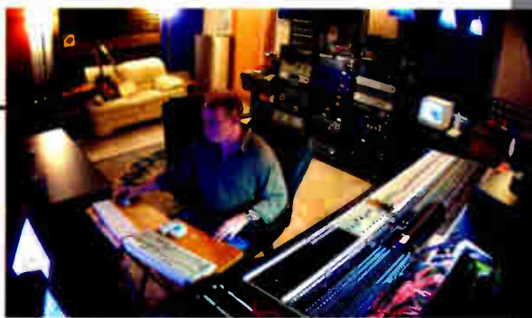
Stuart Sullivan tweaks a mix at Wire, which offers an API 32x12x32 console with Uptown Moving Faders automation, Pro Tools|HD3 Accel and numerous outboard boxes, mics and instruments, all tied to a 16x27-foot main room with four iso booths.
