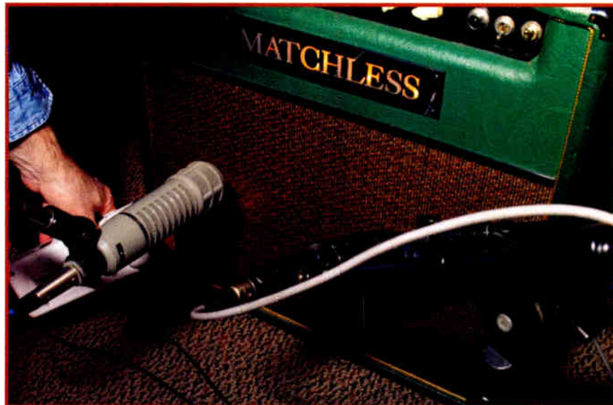
Miking each driver in a dual-speaker cabinet leads to more tonal options in the mix.
