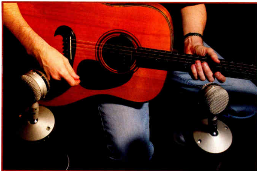
On acoustic guitar, try various spaced-pair mic locations for tonal variety.
