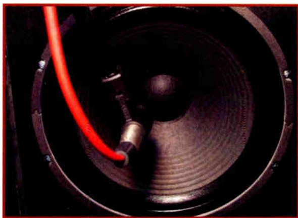
When miking an amp's speaker cone, orient the mic slightly off-center.
