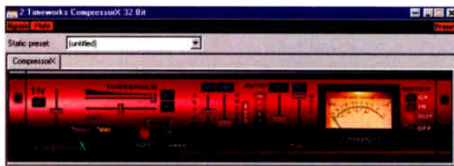
Sonic Timeworks CompressorX employs true stereo 64-bit processing.
