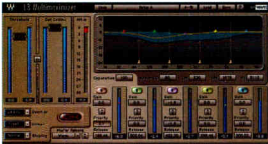
Waves L3 Maximizer: a multiband limiter with phase linear EQ
