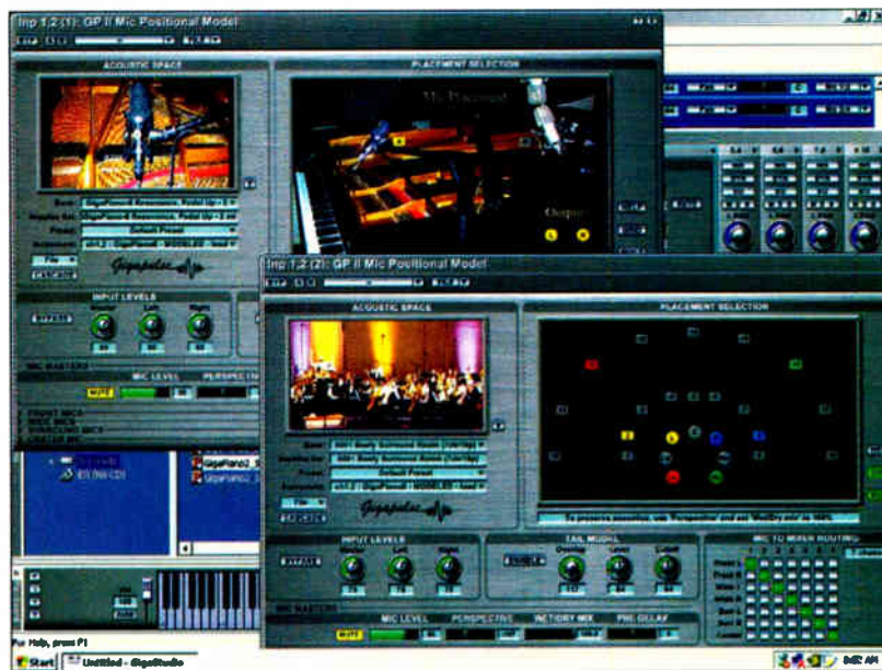
Flexible mic "placements" in GigaStudio 3's GigaPulse provide more variation in sample playback.
