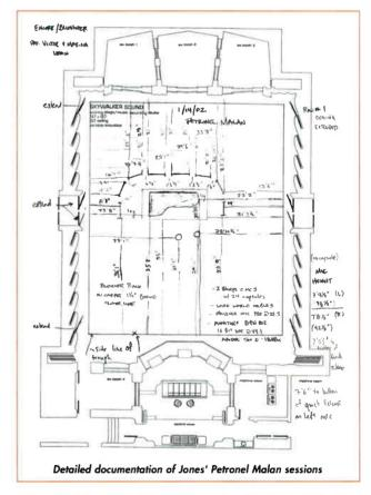
measured and documented. As you can see, the edge of each of the gobos and the position of the piano legs were measured from two walls so they could be positioned exactly if the setup was broken down. The same sheet contains info on the height of the mics from the floor, in this case to the capsule (931/2 inches on the left and 921/8 inches on the right) and another measurement to the quick release.
