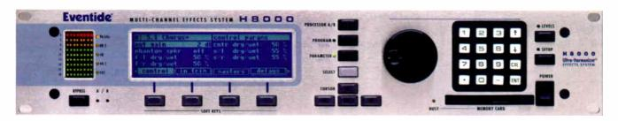
eight AES/EBU, eight ADAT, two S/PDIF and two balanced analog (20 ins and outs total). The analog ins are on XLR/TRS combo jacks, while analog outs are on XLRs; all AD/DAs are 24-bit. All analog I/O can accept unbalanced lines if the cold (pin 3 or ring) signal is shunted to ground, making the H8000 plug-and-play with instrument inputs. (The H8000 can accommodate both line and instrument levels via its pre-A/D boost/cut capability
