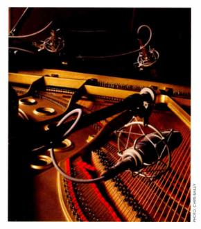
Figure 1: Adding a third mic to a stereo pair can help capture the piano's low range.
