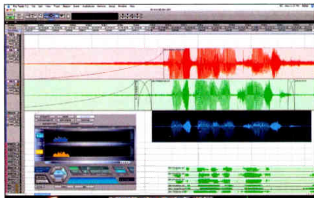
Pro Tools session using VocALign. The red track is the original production dialog; the green track is a production alt take; and the blue waveform is a VocALigned version of the alt track.
