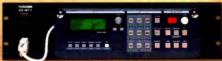
Tascam DS-M7.1 supports LCRS up to 7.1, with downmix capability to mono/stereo.
