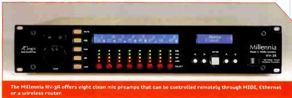
The Millennia HV-3R offers eight clean mic preamps that can be controlled remotely through MIDI, Ethernet or a wireless router.
