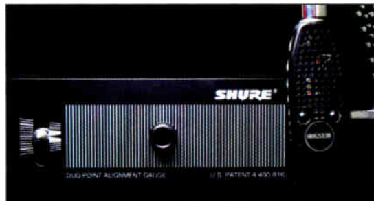
Figure B: Shure's overhang tool has a saddle for its V-15 Series cartridge to snap into; alignment errors are magnified at the spindle.
