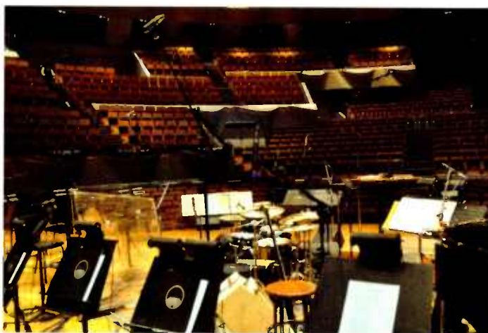
Although there were close to 100 mics onstage, about half of those were used for the eventual broadcast in DTS 5.1; the others were used for SR in the hall.
