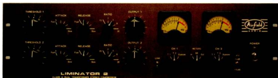
The Liminator 2 features switchable Sowter or Jensen input transformers.
