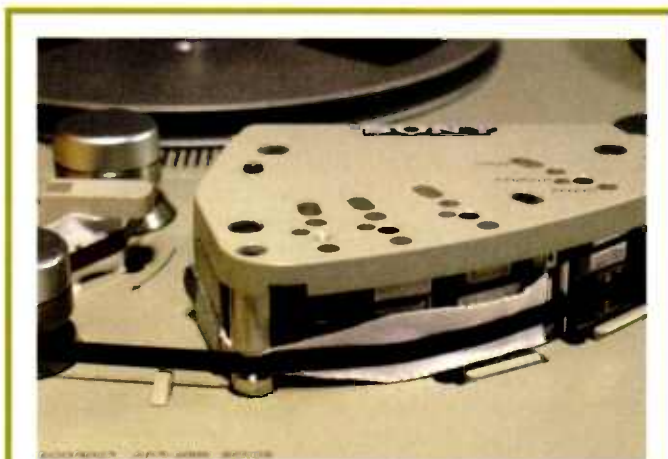
Figure 1: A tape is being “played” while in contact with a porous cloth placed around the tension arm (top-left) and across the heads (center). This technique is used to confirm baking success and remove residual “debris” that might clog the head during playback/transfer.
