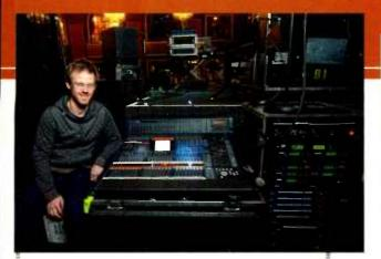
Monitor engineer Colin Burrell mans a Yamaha DM2000, using external A8R preamp/A/D converters for extra inputs into the board, and Aviom A16R and Squirrel Labs Defibrillator. "The band is on in-ears, with no wedges or sidefills," Burrell says. "We're using a Sennheiser IEM system that is greatsounding and very reliable. Some of the band is on ACS ears; others are on Ultimate Ears. I stuck with which models they were using when I started as everyone was happy already."
