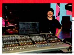
Monitor engineer Neil Taylor also prefers a Yamaha PM5D, but has manned an Avid Profile, Soundcraft VI and a Yamaha M7CL. "I'm using onboard software. The €Q, dynamics and processing work fine, but with the 5D, an external clock makes an incredible difference to the sound and performance of that desk. An Apogee Big Ben is your best friend if you find yourself on a 5D."
