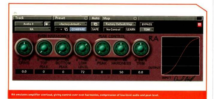
RA is a TDM (only) plug-in from Crane Song's Dave Hill that allows for the manipulation of the ideal linear-transfer function of a virtual amplifier. Running in Mac (and coming to PC soon) Pro Tools hosts only, RA provides four different sections to precisely add generated even and odd harmonics and other distortion artifacts typically brought on by an amplifier overdriven into nonlinear operation.
