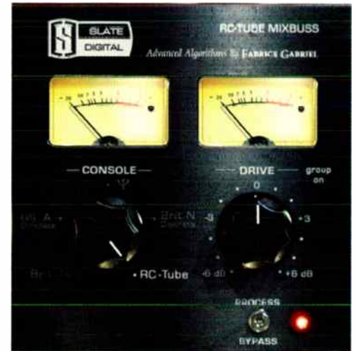
The Mixbus plug-in selects up to four modeled-console stereo mix buses that can be further adjusted with the Drive control.
