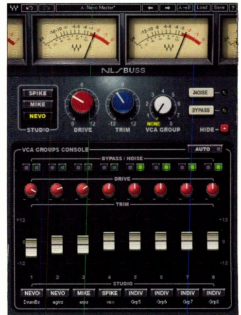
Fig. 2: NLS Buss with the VCA Groups Console display showing in the bottom half of the GUI.
