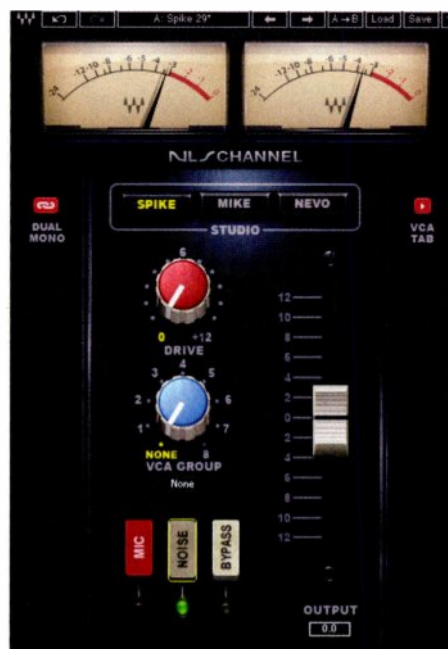
Fig. 1: NLS Channel lets you choose the console type, channel model, mic- or line-input selection, drive amount, output gain and VCA group.
