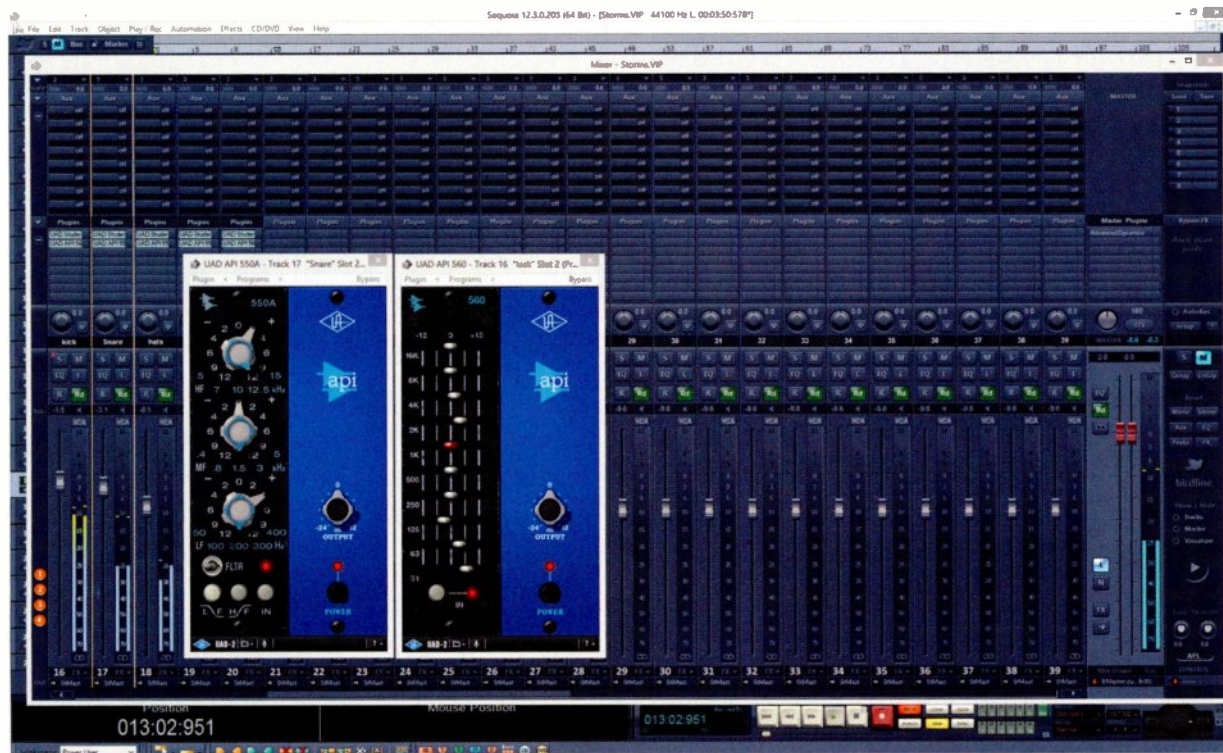
Figure 1: These plug-ins accurately model API's legacy 550 and 560 EQs, including the signature API electronics.
